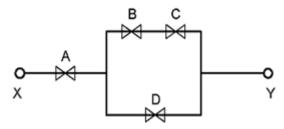
Calculate the probability that flow will not occur between X and Y when a signal is sent to all valves to open, given that valve failures are statistically independent and the probabilities of failure of individual valves and their actuators are
