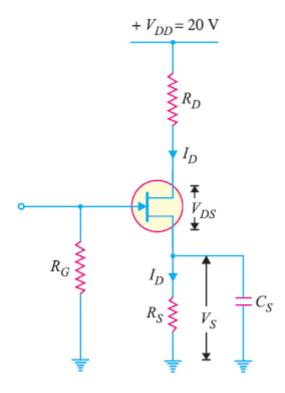
b. Find  $V_{DS}$  and  $V_{GS}$  in Figure below, given that  $I_D = 5mA$  (10 marks)
