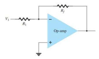
d. Calculate the output voltage  $V_o$  from the circuit of Figure below for an input of 120 mV (3 Marks)
