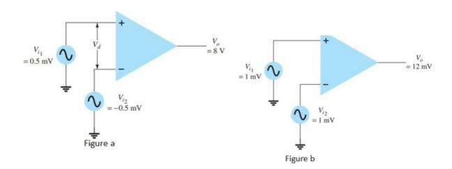
c. Calculate the output voltage for the circuit of Figure. The inputs are  $V_1 = 50mVSin(1000t)$  and  $V_2 = 10mVSin(3000t)$  (05 Marks)
